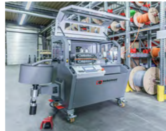
Fig. 4 AUTOCUT 40 with open protective cover
