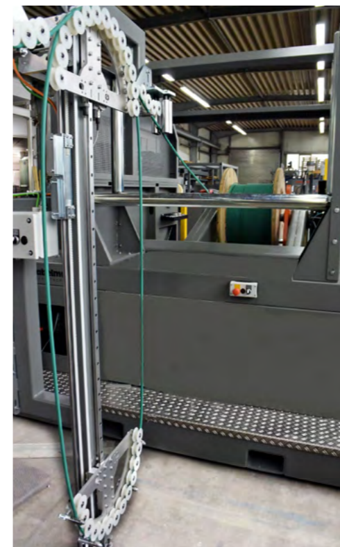
Fig. 2 ACUMATIC: material accumulator / dancer for controlling and synchronization of the drive of the drum. Necessary for tension sensitive winding goods.
