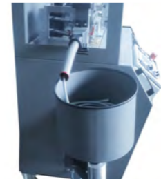
Fig. 5 Pot winder with adjustable drive motor
