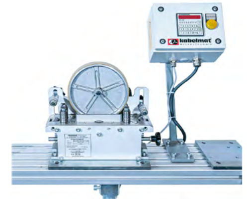
Fig. 2 MESSBOI 40 LC with counter in housing
