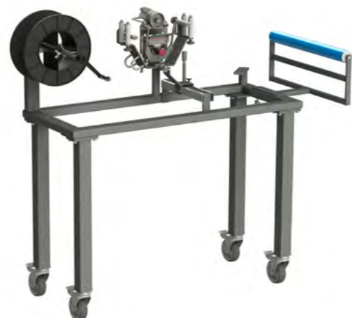
Fig. 2: MESSROL 450 with spool winding axle, MESSBOI 25 with roller cage unit and inlet roller
