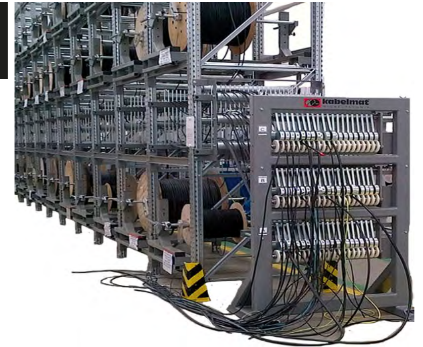
Fig. 2 TROMBULLY with central point of removal and return stop
