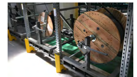
Fig. 3 TROMTRAK 1000 drum storage device in use
