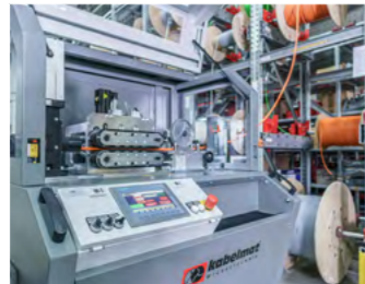
Fig. 3 Control panel with touch panel control and regulated positioning servo drive
