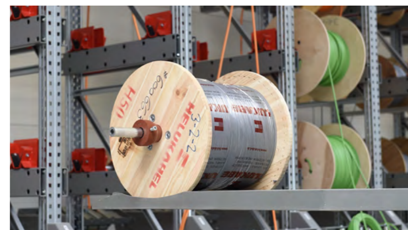
Fig. 2 TROMPLAT 1000 example of storing the drum into a Kabelmat LAGROL rack
