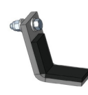
Fig.13 Brake pad for axle drum Ø60 mm
