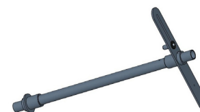
Fig.16 Drum axle incl. driving pin
