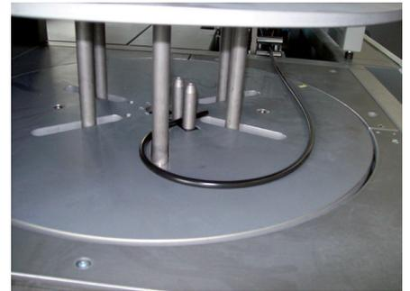
Fig. 4 Cable fixing clamp for winding plate
