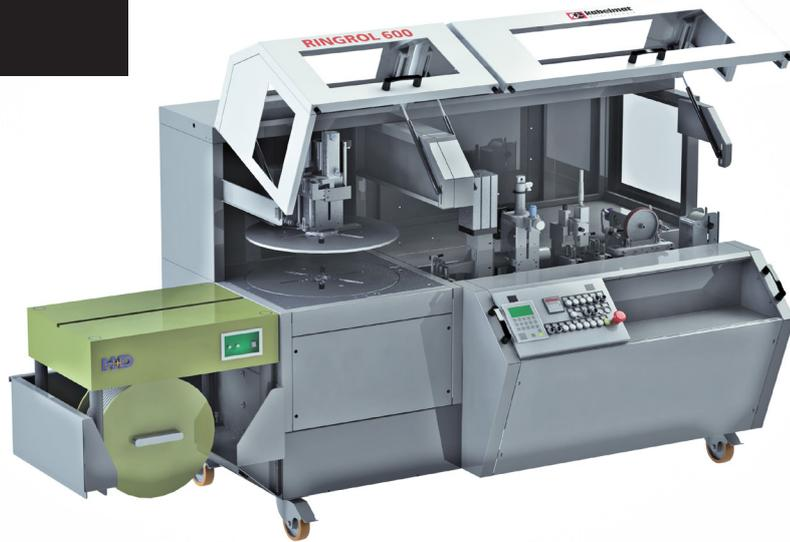
Fig. 1 RINGROL 600 with open cover and binding device
